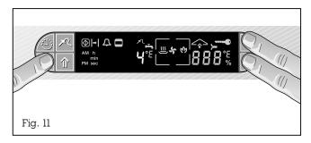
If the hardness of the water in your household deviates from the value that is set at the works (water hardness range 4), you must enter the right water hardness in the options menu for commencing operation of the appliance.
